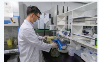
Concentrating viruses in wastewater to detect their RNA
